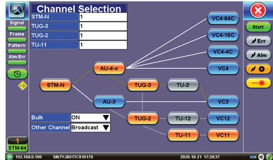
PDH/DSn client can be multiplexed and mapped into SDH/SONET.
